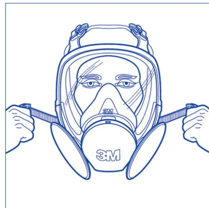
2. Pull the ends of the four straps to adjust tightness, starting with the neck straps first, then the forehead straps. Do not over tighten the head straps.
