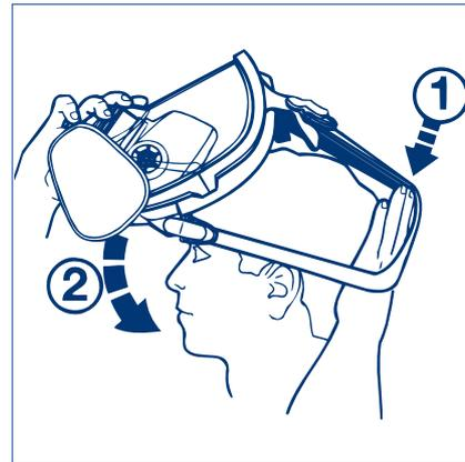
1. Fully loosen all four head straps, then place the harness at back of head and position facepiece over the face.
