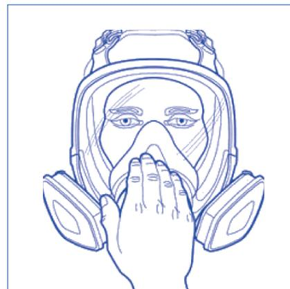
3. Perform a positive and/or negative pressure fit check each time the respirator is donned.
